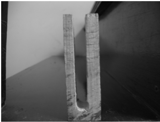
Fig. 10: Photograph of parawood after the prong test
